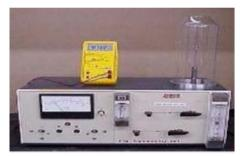
The test is performed in accordance with the procedure specified in ASTM 2863-95 using test piece cut from the outer sheath of the cable. The apparatus holds a small specimen which is clamped vertically in a tube in an atmosphere where the relative concentration of oxygen and nitrogen can be changed. The aim is to test the flammability of the sample with a small pilot flame to find the minimum oxygen concentration required to just sustain combustion of the sample.
