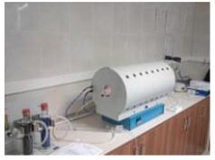
50267-2-3:1999 (CEI 20-37/2-3). Common test methods for cables under fire conditions- Test on gases evolved during combustion of materials from cables- Part 2-3:Procedures. Determination of degree of acidity of gases for cables by determination of the weighted average of pH and conductivity.
